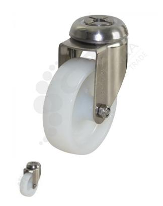
nylon wheel. This swivel castor is part of our stainless steel elite bolt range and can safely take loads up to 100kg. The S4490 uses plain bearings for wheel rotation and is mounted with a bolt. The swivel frame of this castor permits the load to be steered. The nylon wheel diameter is 100mm, the wheel width is 30mm and can be ordered separately (NY4417). This model can also be ordered with a brake (part number S4490B).
